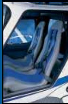
aluminum crush elements and memory foam in critical areas, exceeding the latest FAA standards.
